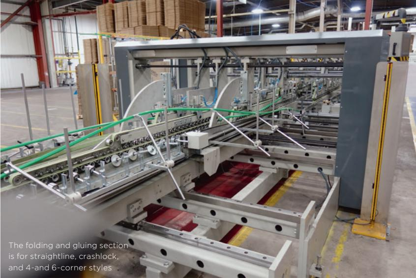
The folding and gluing section is for straightline, crashlock, and 4- and 6-corner styles
